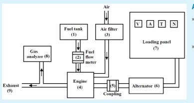
Image: Schematic diagram of the Set-Up
